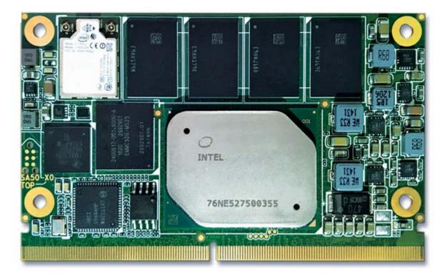
For example, the credit-card-sized conga-SA5 SMARC 2.0 modules *(example shown above)* are available with either the <u>Intel</u> Atom processors x5-E3930, x5-E3940, or x7-E3950 for the extended temperature range –40 to +85°C, or with the Intel Celeron N3350 or quad-core Intel Pentium N4200 processors.
