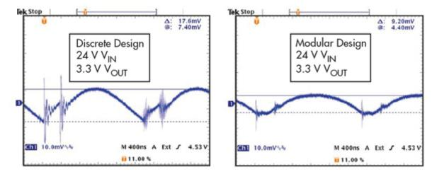
*Figure 4* compares the output noise performance of the discrete and modular designs. The LMZ14203 stacks a shielded inductor on top of the controller in a three-dimensional package to minimize trace length and inductance.
