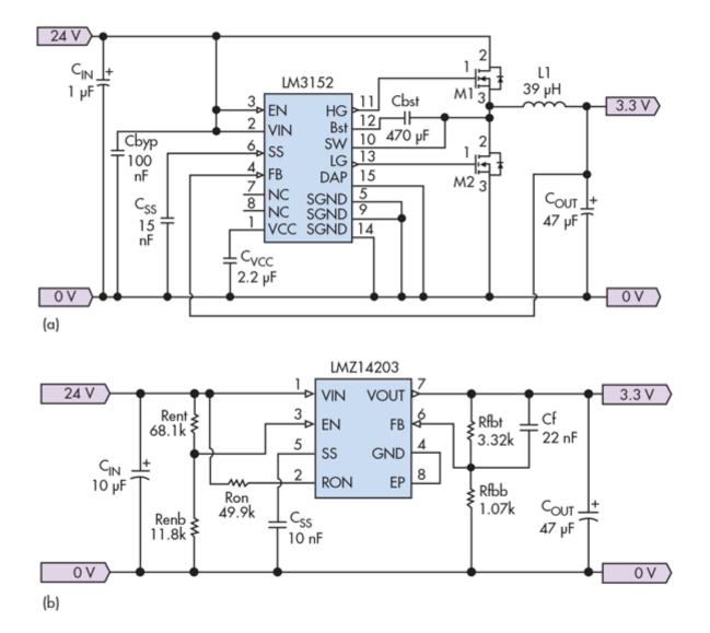
h designs used the WEBENCH tool to develop the schematic and select the external components. Each design d 10 components in total, but there were significant cost differences. The modular design required only \$0.69 of resistors and capacitors, but had an estimated total BOM cost of \$10.19; the discrete design needed \$1.69 of external components including resistors, capacitors, an inductor, and two FETs, but its estimated total BOM cost was only \$4.14.
