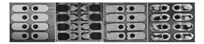
To achieve the desired soldering effect, an appropriate amount of tin paste should be maintained on each through-hole pad of through-hole mounted components to supplement the solder. Otherwise, it will cause defects such as an insufficient amount of tin inside the through hole, a void, or bubbles.
