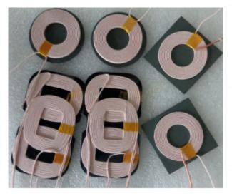
Transmitter and receiver coils are typically constructed from <u>Litz wire</u>; this consists of many insulated strands wound in a specific pattern to minimize the skin effect and reduce proximity losses. For higher power levels, the coil is mounted on a sheet of ferrite. A manufacturer of transmitters and receivers often <u>publishes a list</u> of recommended coils for use with its products.
