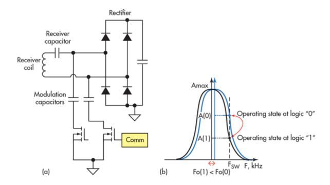
The communication scheme is digital, with packets being transferred from the secondary to the primary. The Qi standard specifies a data rate of 2 kb/s with biphase bit encoding. A variety of communication packets have been defined for functions such as identification and authentication; error detection; control; power usage; end of power; and efficiency.
