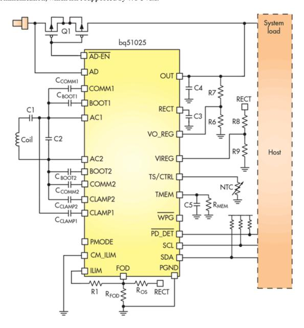
The bq51025 features adjustable outputvoltage of 4.5 to 10 V, and enables a system efficiency of up to 84%. The I<sup>2</sup>C interface allows for easy interfacing to a low-power microcontroller, such as one of TI's MSP430 family.
