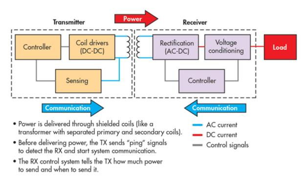
During operation, the transmitter is in a low-power "snooze" mode most of the time and wakes up periodically to check whether a receiver is present. If it detects the presence of a secondary coil, the transmitter requests authentication from the receiver. After a successful authentication the transmitter initiates charging; otherwise, it goes back to sleep (*Fig. 1*). The secondary side maintains full control over the power transfer using communication packets.
