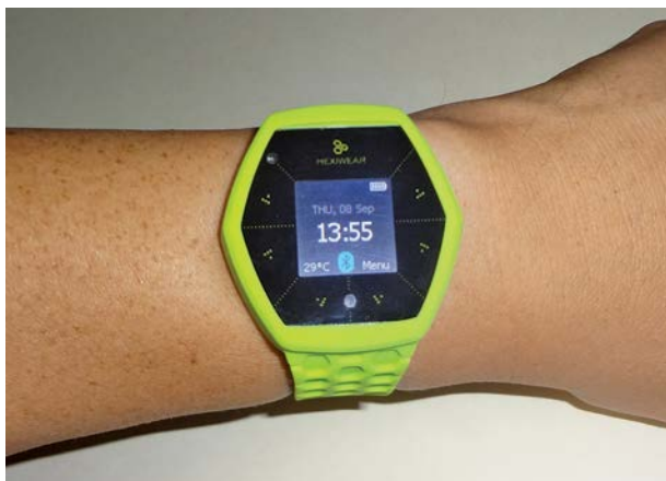
1. The Hexiwear module can fit into a wristband. The heart-rate sensor is on the back of the module.
