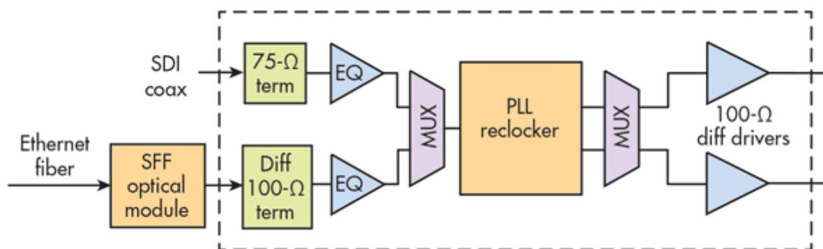
Designing transmitting and receiving circuits requires special circuits to correct for these limitations. Amplification overcomes attenuation, while an equalizer at the receiver can correct the distortion based on cable length. Jitter can be corrected by reclocking the data stream. Special integrated circuits are available, making it unnecessary to design them yourself.
