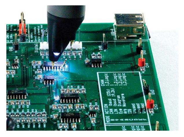
For example, at 75 MHz, the passive probe's capacitance will present a 150- $\Omega$  impedance to ground, while the active probe's capacitance will present a 2.5-k $\Omega$  impedance to ground. The smaller capacitance of the active probe will result in less loading of ac signal content above 10 kHz versus the passive probe.
