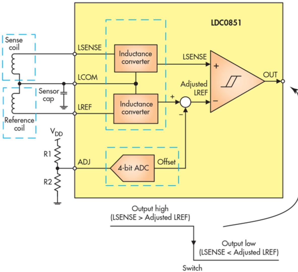
In general, the output switches low when the sense inductance drops below the reference and returns high when the reference inductance is higher than the sense inductance. Switching occurs during the crossover point when the two inductances are equal.
