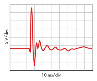
The silicone adhesive allows a rubbing notion when the assembly is tapped from above or on end, as shown by the arrows. The generated charges are collected by the metal tine and the copper surfaces of the circuit board. When discharged into a large resistance, impressively high voltages can be generated *(Fig. 2)*. (The author's demonstration switch was four inches long and 3/4-inch wide, but smaller switches are possible.)
