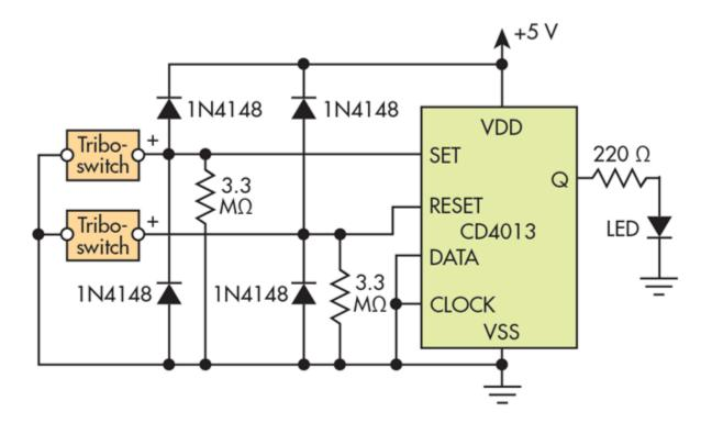
You can use such switches to activate CMOS digital circuitry *(Fig. 3)*, where two triboelectric switches control a set-reset flip-flop and control an LED. The diodes prevent high voltages from damaging the input transistors of the <u>CD4013</u> integrated circuit.
