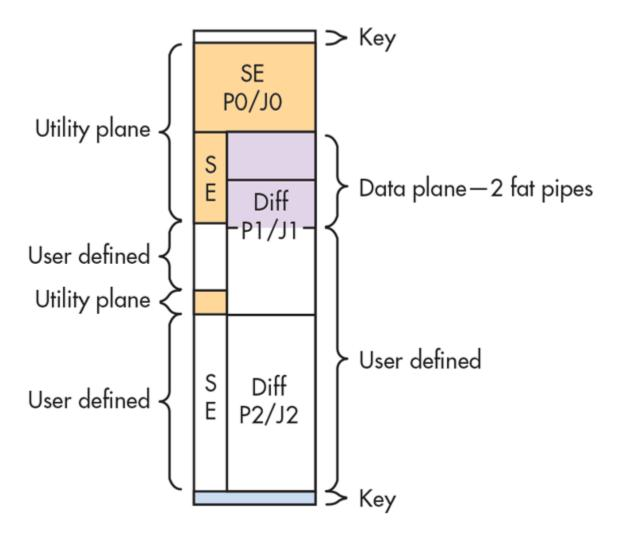
The *Slot Profile* defines the connector type and provides a physical mapping of ports onto a given slot's backplane connectors. *Figure 1* shows a Slot Profile of a slot in a 3U VPX backplane.
