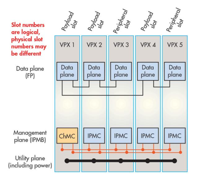
The Backplane Profile shows a physical definition of a backplane implementation and the topologies used to
