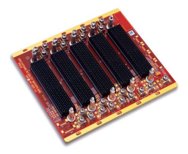
OpenVPX added a couple of other minor changes to the backplane. This includes redefining two reserved PO/JO signals Aux\_Clk (+/-), redefining the Res\_Bus signal to GDiscrete, and adding one P1/J1 single-ended utility signal of Maskable Reset. The Aux\_Clk and GDiscrete pins were previously bussed anyway, so the change is negligible. The SysCon signal also became configurable with OpenVPX.
