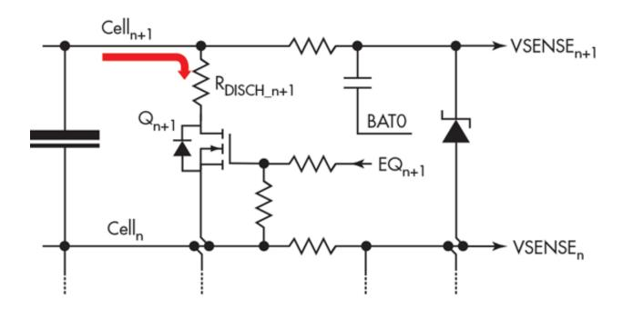
The control algorithm, running on the BMS microcontroller, balances the charge in each cell by measuring its voltage VSENSE and discharging the cell if necessary until all cells are at the same voltage. The BMS also checks for battery-level fault conditions such as overtemperature, overvoltage, and undervoltage. Once all cells are balanced, the battery pack as a whole can be charged to fully charge each cell.
