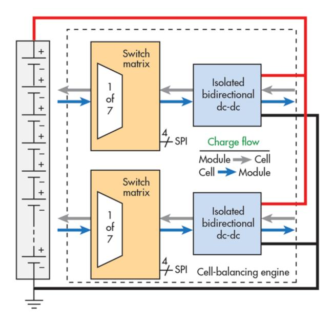
Figure 5 shows a block diagram of a typical active load-balancing engine.
