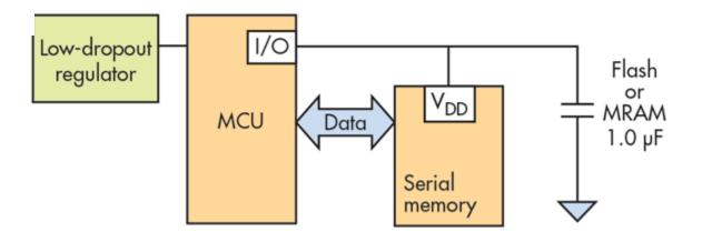
The MCU was assumed to be in a low power sleep state and with a periodic wakeup for data acquisition. The data acquired was stored in the non-volatile memory, and then the system returned to the sleep state.
