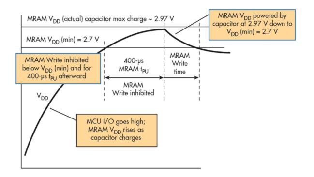
*Rise time:* During this phase, we assume that all of the energy goes into the decoupling capacitor and that the non-volatile memory consumes negligible energy.
