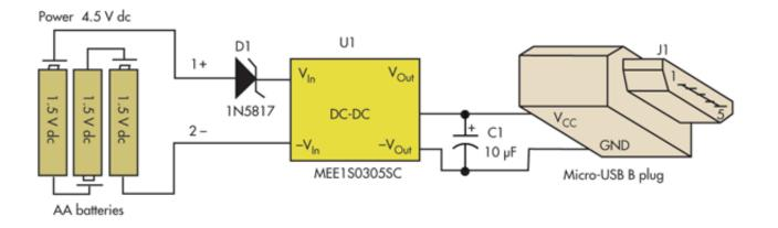
There are many different standard AA batteries *(Table 2)*. In the 3-unit AA battery holder, the batteries are connected in in series to produce4.5 V for the regulator. Note that lithium-ion batteries don't need to be in series. They can all be in parallel. *Table 3* reviews some available cell phones along with their battery capacity. Do NOT mix battery chemistries!
