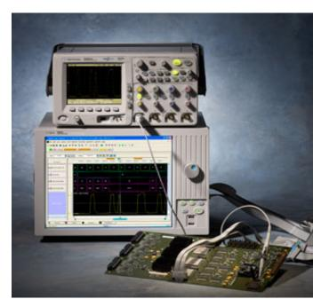
2. Logic analyzers uniquely offer both state and timing analysis. State analysis enables the capture of longer time windows and filters out transitions between valid states. Logic analyzers can interact with scopes when cross-triggering capabilities are needed. And, time-aligned scope waveforms can be imported into the logic analyzer viewer as shown here with Agilent's 16800 logic analysis system.
