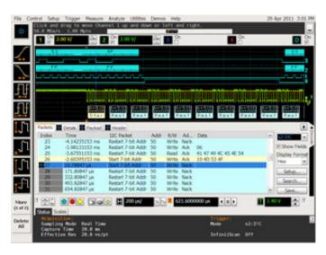
3. MSOs typically include power options for serial bus triggering and decode. In this example, two analog channels were used to capture and decode I2C while four MSO digital channels were used to capture and decode SPI.
