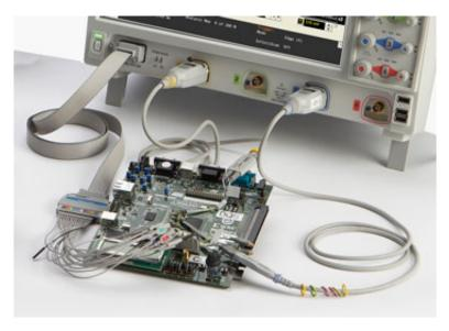
1. The digital channels in MSOs add incremental debug capability to scopes, as shown here with Agilent's Infiniium 9000 series oscilloscopes. MSOs excel at low-speed serial bus triggering and decode. They also enable triggering across both analog and digital channels.
