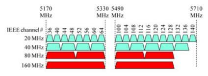
4. Data channels for 802.11ac in Europe are similar to the U.S. channels, but with different frequency assignments.
