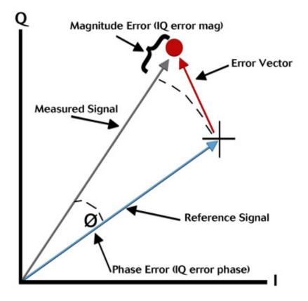
6. Vectors represent the amplitude and phase of the carrier to illustrate EVM. The reference standard signal is compared to the measured signal. An error vector and phase error provide the EVM measurement. The error magnitude is expressed in dB compared to the vector amplitude.
