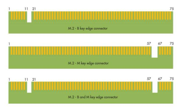
While a motherboard can incorporate a range of key M.2 socket options, the most popular are B and M *(Fig. 1)*. The B interface provides x2 PCIe, SATA, USB 2.0 and 3.0, audio, UIM, HSIC, SSIC, I2C, and SMBus support.
