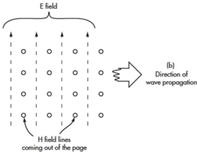
2. At a distance from the antenna, the E and H fields are essentially planar and intersect at right angles. Note the direction of propagation, which is perpendicular to both fields. At (a) the direction of propagation is perpendicular to the field lines shown either into or out of the page. In (b) the magnetic field lines are coming out of the page. You can picture them as lines with arrow points shown as dots.
