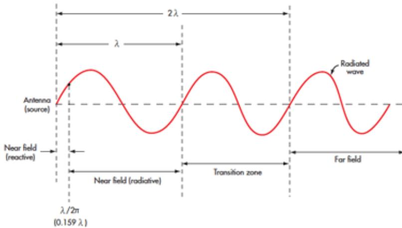
3. Boundaries of the near and far fields are shown with respect to wavelengths at the operating frequency.
