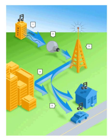
1. The HD Radio process begins with the station combining the analog and digital audio signals with text (1). It then compresses the digital signals using iBiquity's compression technology (2) and sends the package of signals to the transmitter, where the broadcast occurs (3). The signals undergo some interference and multipath fading, minimized by the HD process (4). Finally, the signals are received at vehicle and home radios (5). (courtesy of iBiquity Digital Corp.)
