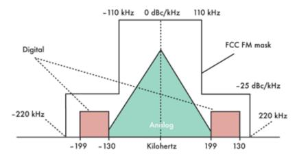
3. The standard analog signal in the FM band is within a 260-kHz bandwidth with digital sidebands outside the ±130-kHz limits. Modulation is OFDM with QAM. The FCC mask shows the spectral limits allowed.
