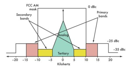
2. The standard analog signal in the AM band is within the normal 10-kHz bandwidth, while the digital spectrum is above and below the ±5-kHz limits. Modulation is OFDM with QAM. The FCC mask shows the spectral limits allowed.
