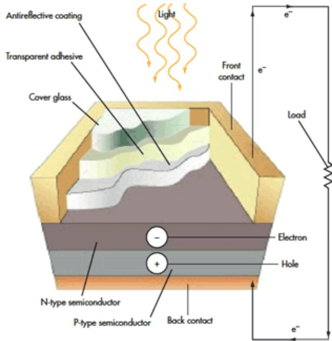
1. One example of a crystalline silicon cell consists of seven material layers, two of which - the outer electrical contact - hold the entire package together.
