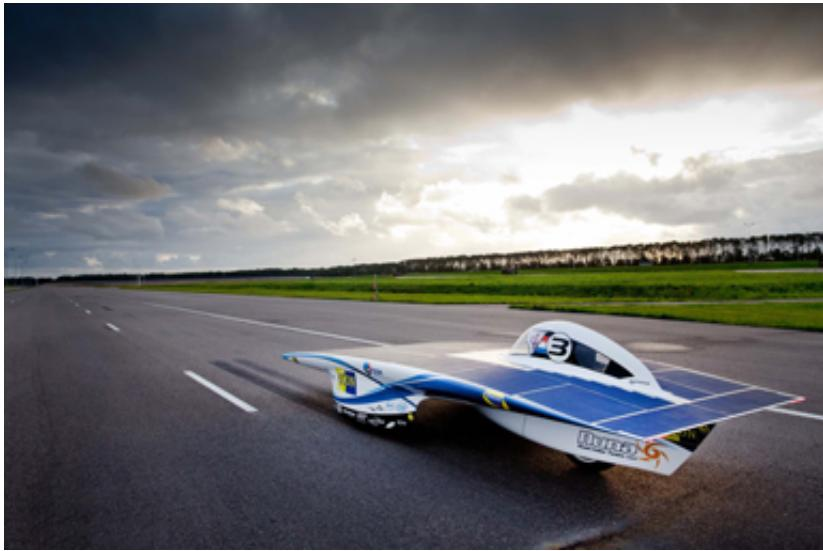
4. Extending the Nuna series of solar-powered cars, the Nuna 6 spreads 1690 monocrystalline silicon solar cells over its body. The cells work with a 21-kg Li-ion battery and deliver an efficiency of 22%.
