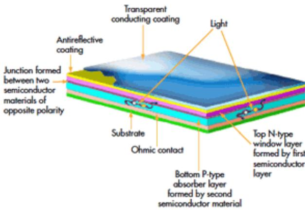
2. Consisting of six layers in this case, a thin-film solar cell is not much different in construction than its c-Si counterpart and operates on the same photovoltaic principle.
