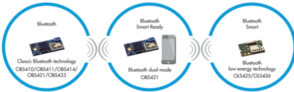
2. Complete Bluetooth modules developed by connectBlue include a classic Bluetooth module, a Bluetooth Smart Ready module that supports both standard Bluetooth and BLE, and a Bluetooth Smart module that includes only BLE.
