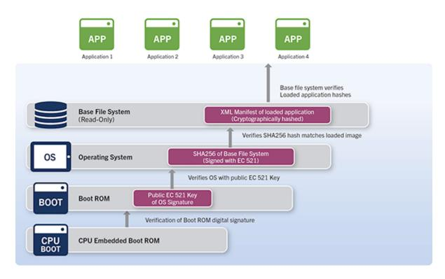
Securing the boot process can come with tradeoffs, including lower performance. It will take longer for a system to boot in a secure fashion. Why? Because the system must follow a number of steps to ensure the boot process is in fact secure *(Fig. 1)*. For example:
