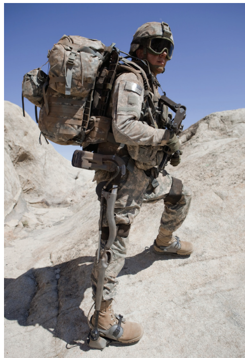
3. The HULC (Human Universal Load Carrier) uses hydraulics to provide heavy lifting capabilities.
