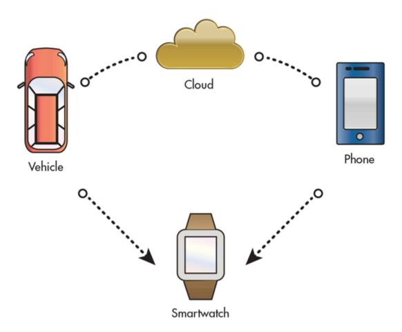
Thanks to near-field communication (NFC), a proximity technology enabling communication between devices, it's easy to identify and configure a driver's or passenger's preferred settings. Though the capabilities of a smart watch are rather restricted when it comes to changing settings, it's a convenient tool for information storage and notifications. Detailed settings may be changed via a connected mobile device or automobile media system connected with the Internet.
