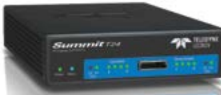
2. Teledyne LeCroy's Summit T24 Protocol Analyzer can handle new protocols such as NVMe.
