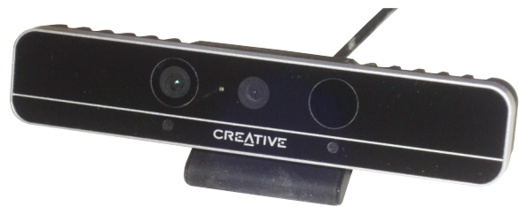
Intel's RealSense SDK, which features an extensible plug-in framework, targets Creative Technology's latest F200 3D camera.
