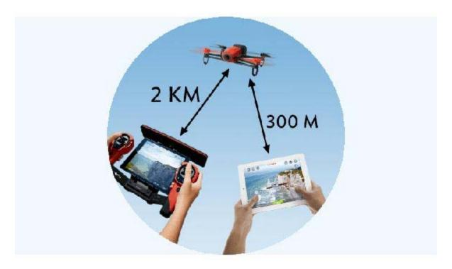
**Loury:** The Bebop Drone Skycontroller *(Fig. 2)*, an RC-like remote control equipped with a Wi-Fi amplifier powered by an amplified Wi-Fi radio and four antennas, provides an even more powerful Wi-Fi connection. The piloting smartphone or tablet is fixed on the control dock and streams what the Bebop Drone is seeing on its
