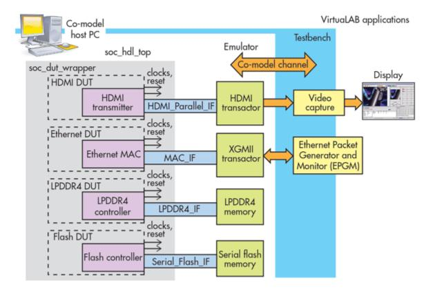
The environment is a software implementation of in-circuit emulation (ICE) applications, where the design under test (DUT) is driven by the OS (e.g., Linux or Windows) using drivers, applications, and software stacks. This approach avoids the creation of hardware-verification testbenches (SysVerilog, for instance) not understood by software engineers. As a result, designers can create scenarios and environments well understood by software engineers.
