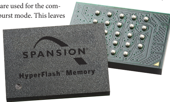
2. Spansion's HyperBus NOR memory is available in 8 mm by 6 mm packages with up to 512 Mbits of storage.
