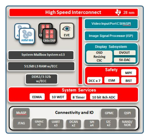
In typical applications the chip uses 1 to 2 W of power. It is available in 15- by 15-mm and 12- by 12-mm chips with package-on-package (PoP) support. This support allows integration with a range of third party LPDDR2 memory chips although for some applications the on-chip memory may be sufficient. Versions are available
