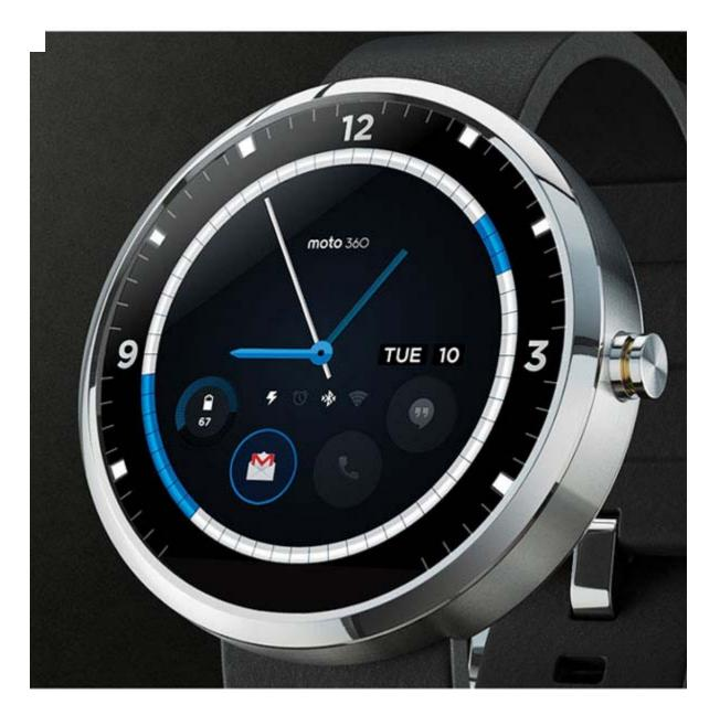
The Moto 360 as a 1.56-in backlit color LCD display with a resolution of 320- by 290-pixels (205 ppi). The display is more demanding in terms of power compared to an e-paper display but it provides a more colorful display. This allows features like a background that reflects weather to alerts with sophisticated animations.
