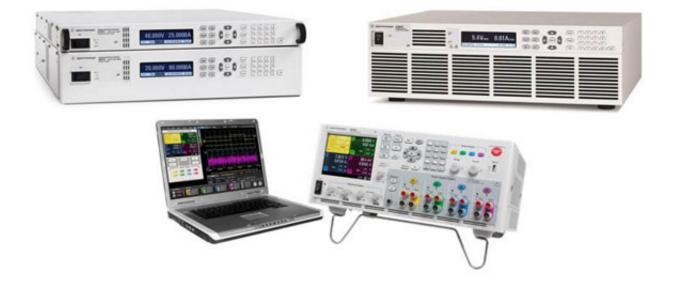
The built-in watchdog holds several advantages over the custom circuit. It requires no additional design or maintenance. It's simpler to interface to the system, requiring no additional hardware or wiring. Lastly, the watchdog is simpler to control, because the watchdog is programmed like any other feature of the supply. Figure 2 shows various examples of power supplies with built-in watchdog timers.
