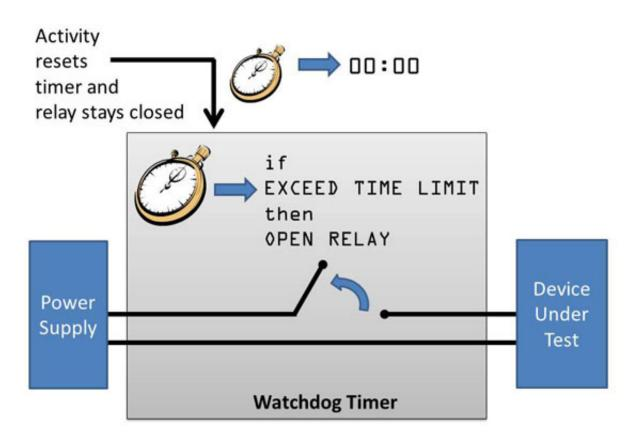
Under normal conditions, when powering (via ac or dc power supply) your device during an automated test, some specific activity occurs within the test system. In turn, the watchdog timer restarts so that it won't elapse, or "time out." If, due to a hardware fault or program error, activity stops and the watchdog timer fails to restart, the timer will elapse and place the power supply in a safe state to avoid uncontrolled power going to the device under test (DUT) (*Fig. 1*).
