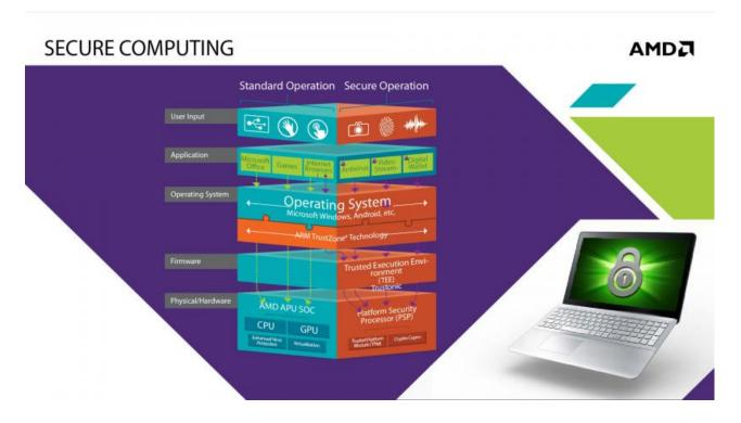
A prominent example of this approach is the TrustZone technology developed by ARM (*see the figure*). This open platform includes programmable software components and applications that enable computer hardware designers to create customized security solutions or counter specific security threats.
