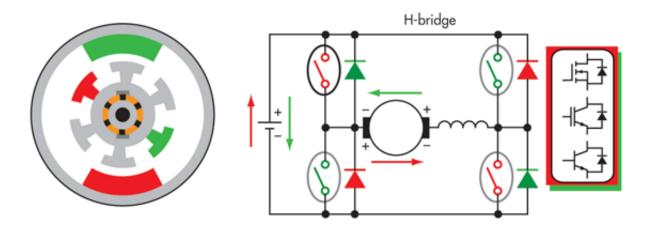
Due to the shortcomings of brushed dc motors, BLDC motors were developed (*Fig. 2*). They offer tremendous advantages, including greater torque, increased efficiency and reliability, and longer lifetimes from a lack of brush and commutator wear. They also eliminate sparking from commutators and reduce overall electromagnetic interference (EMI).
