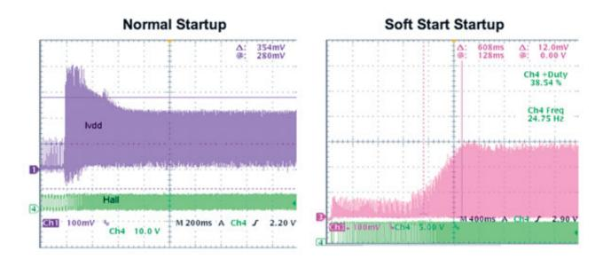
When controlling multiple fans with a single device, inrush current also can be limited by implementing a staggered startup methodology (turn on fan 1 and 2 first, then fan 3 and 4, and so on). By doing this, you allow time for the inrush from the first two fans to settle before the startup of the next two fans, rather than a massive inrush from turning all fans on at the same time.
