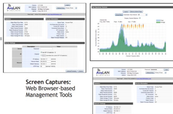
► Figure 5: Sample of web browser-based diagnostics monitoring, link analysis, and remote configuration.
