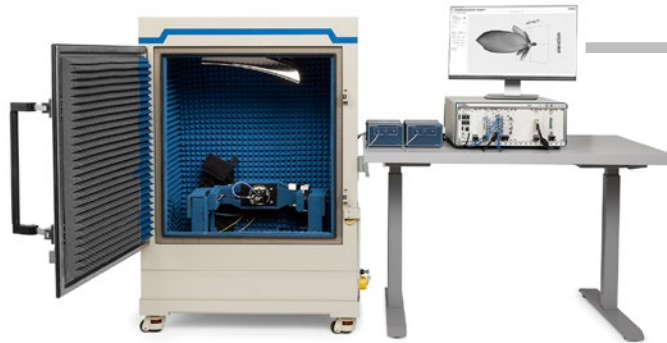
◀ Figure 5: Engineers must make their measurements over the air (OTA) in a controlled RF environment inside anechoic chambers.
