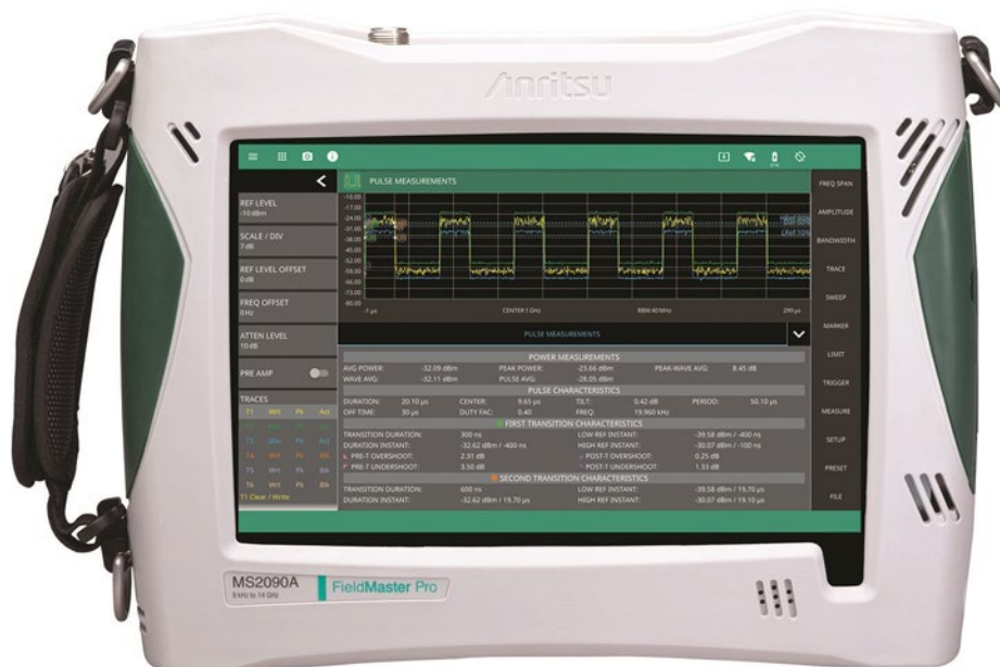
Figure 1: The Anritsu Field Master Pro MS2090A real-time spectrum analyzer has a frequency coverage up to 54 GHz.
