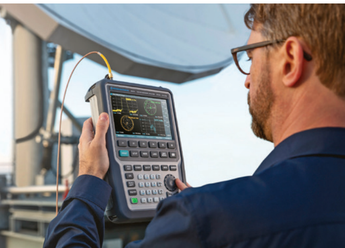
◀ Figure 12: The R&S ZNH handheld 2-port VNA offers 16,001 measurement points.
