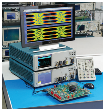
▼ Figure 9: DPO7000SX oscilloscopes can perform BER measurements without the need of an additional instrument.
