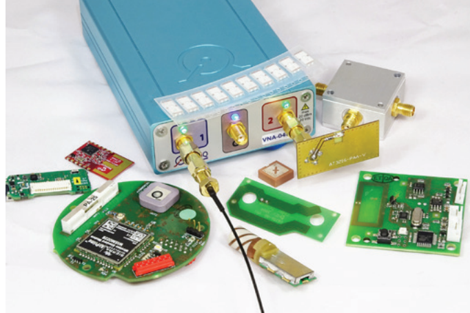
◀ Figure 17: The VNA-0460 is a USB-driven 6GHz 2 port VNA with PC software.
