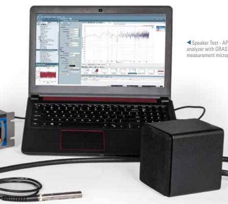
Speaker Test - APx517B analyzer with GRAS 46AE measurement microphone
