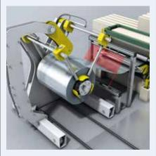
SICK's MLG-2 WebChecker light grid performs high-performance running edge detection, as well as width and center measurement. Used for the processing of web-shaped packaging materials, it is able to detect web width changes or deviations in the web position and report to the follow-up control system of the packaging machine in the same work process with an accuracy of  $\pm$  0.3 mm and a resolution of 0.1 mm per web edge.
