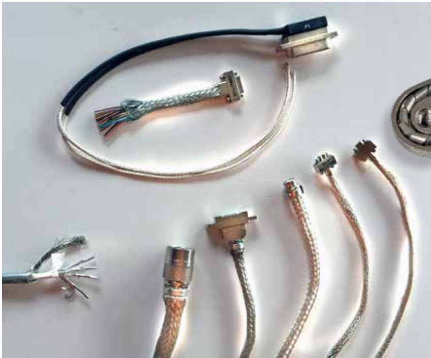
Shielded application-specific wire-harnesses are used in systems where performance and electronic interference is a serious concern. Courtesy of Omnetics
