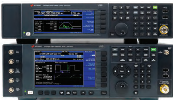
◀ Keysight UXG Agile Vector Adapter (top) and UXG Agile Signal Generator (bottom).
