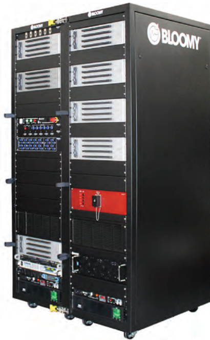
▲ Bloomy Controls FADEC and ECC test platform.
