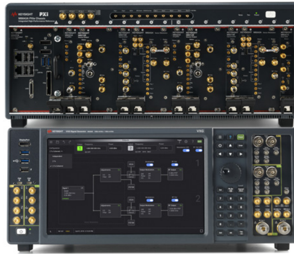
◀ Keysight Technologies VXG microwave signal generators in PXI (top) and benchtop (bottom) configurations.
