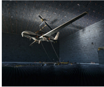
▲ An MQ-4C Triton is lifted inside Patuxent River's (Maryland) anechoic chamber during August 2015 for EMC testing. © U.S. Navy
