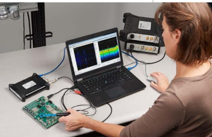
◀ An engineer performing EMI debug troubleshooting a Tektronix real-time spectrum analyzer.
