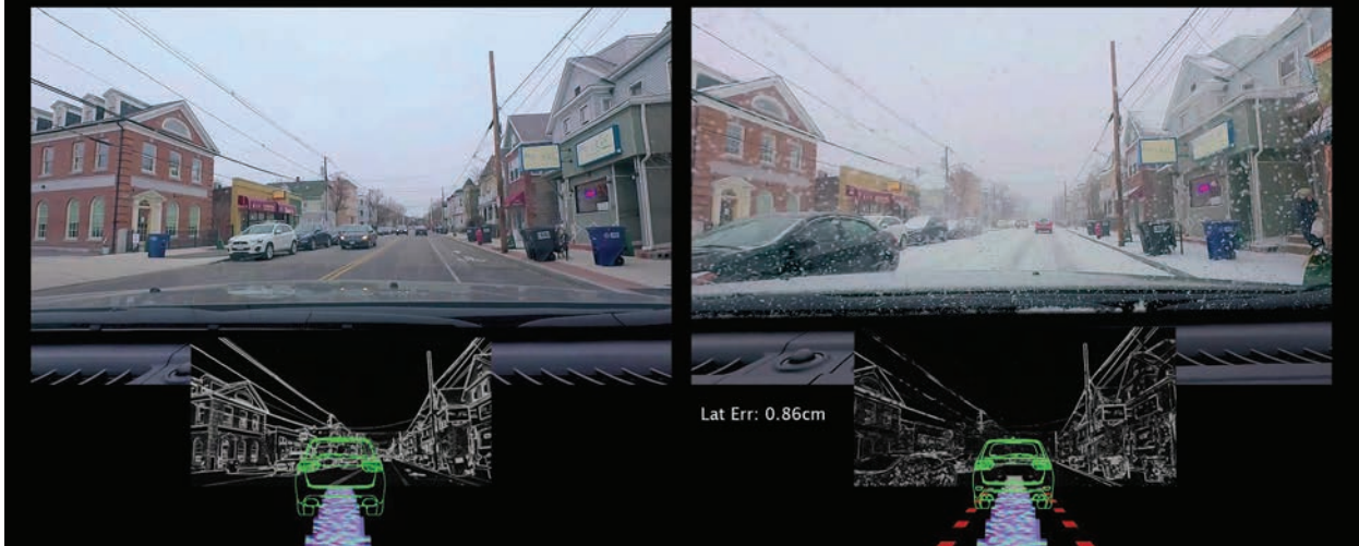
▲ Mapping in clear conditions (left) and tracking in snowy conditions (right).
